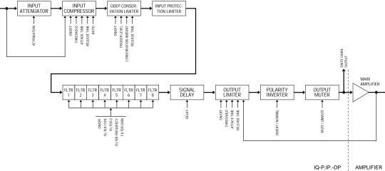
Fig. 5.2 IQ-P.I.P.-DSP Audio Signal Flow Block Diagram
